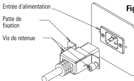
**Figure 1-9.** Cordon de raccordement
